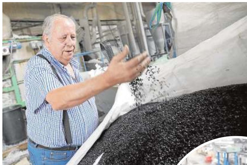
▲ 'Lentils'. Polythene is the raw material used to mould the irrigation piping. :: MIGUE FERNÁNDEZ
