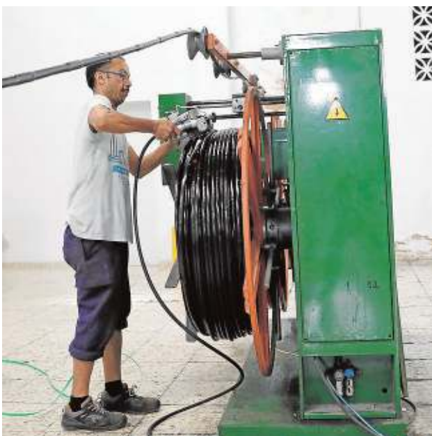
▲ Just made. A worker winds up the tube in the machine. :: MIGUE FERNÁNDEZ
